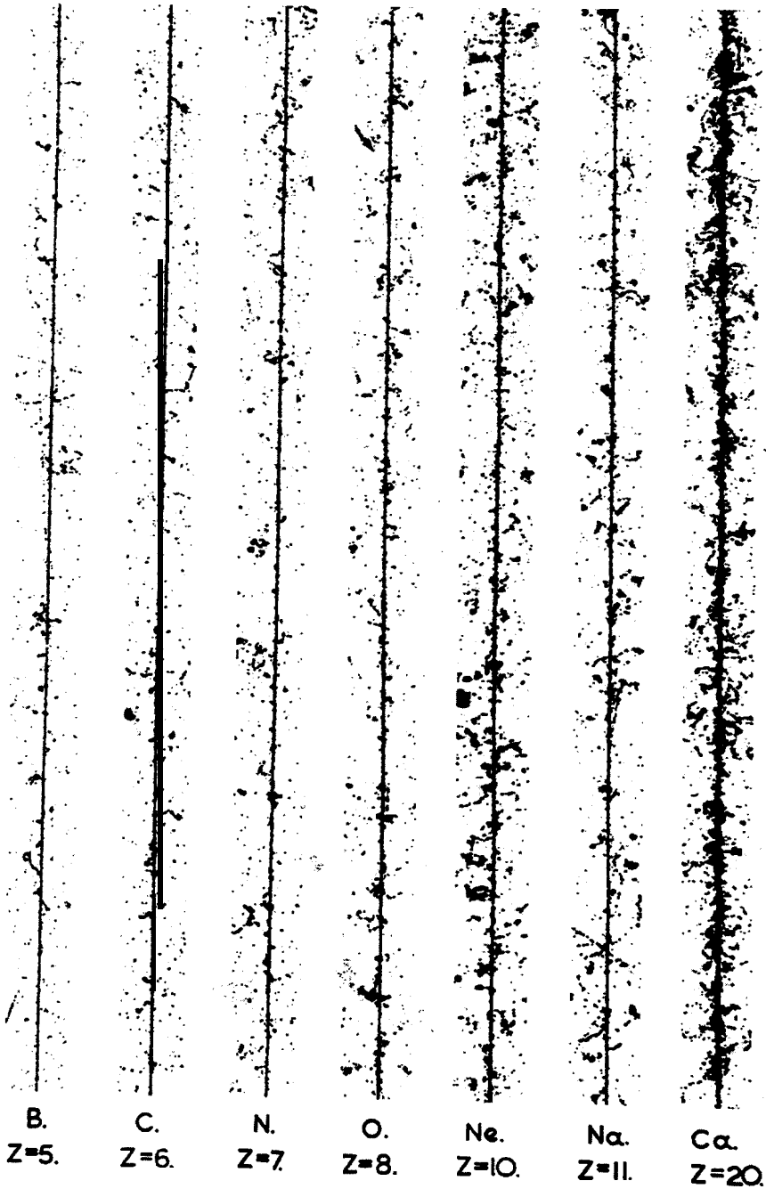
Fig. 2. Examples of the tracks in photographic emulsions of primary nuclei of the cosmic radiation moving at relativistic velocities.
