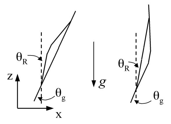
**Fig. 4.** The spatial areas enclosed by the two Ramsey-Bord interferometers due to a misalignment of the Raman beams  $\theta_R$  or the launch  $\theta_L$  with respect to gravity, g. The areas of the two interferometers are equal so that  $\Phi_1$  -  $\Phi_1$  ~ 0.
