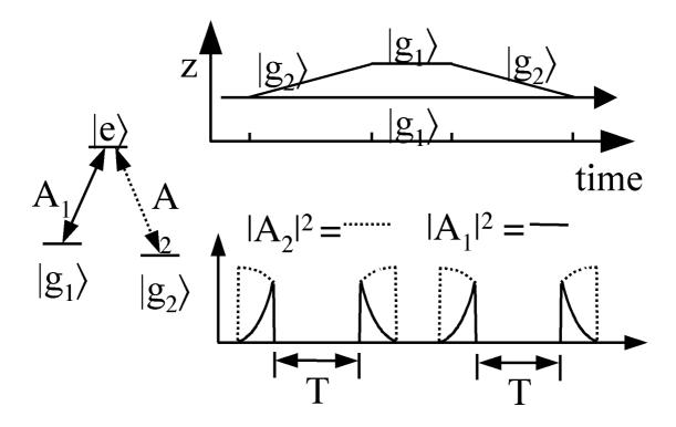
Fig 3. An atom interferometer based on adiabatic transfer between ground states  $|g_1\rangle$  and  $|g_2\rangle$ . The upper diagram is a space-time diagram of the lower interferometer of Fig. 2. The intensity profiles of the pulses used to produce  $\pi/2$  transitions for this interferometer are shown. In order to create the upper interferometer, the shapes of  $A_1$  and  $A_2$  are changed as indicated. In this figure,  $k_1(k_2)$  is directed upward (downward.)
