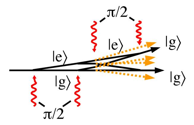
**Fig 2.** A space-time trajectory of a Ramsey-Bord interferometer beginning with an atom initially at rest. Each arrow indicates the direction of the k-vector of the  $\pi/2$ -pulses. The dotted lines show atomic paths that do not contribute to the interference signal.
