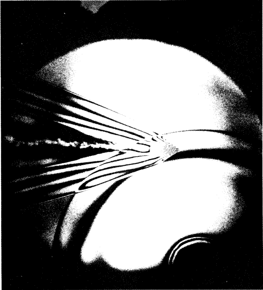
Fig. 17. Dynamic Holographic Interferometry. This Reconstruction of a Holographic Interferogram shows the interaction of two air shock fronts and their associated flows. (Courtesy of Dr R. F. Wuerker and his associates, TRW Physical Electronics Laboratory, Redondo Beach, Calif.)
