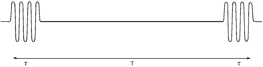
Figure 4. Two separated oscillatory fields, each acting for a time \tau , with zero amplitude oscillating field acting for time T . Phase coherency is preserved between the two oscillatory fields so it is as if the oscillation continued, but with zero amplitude for time T .
