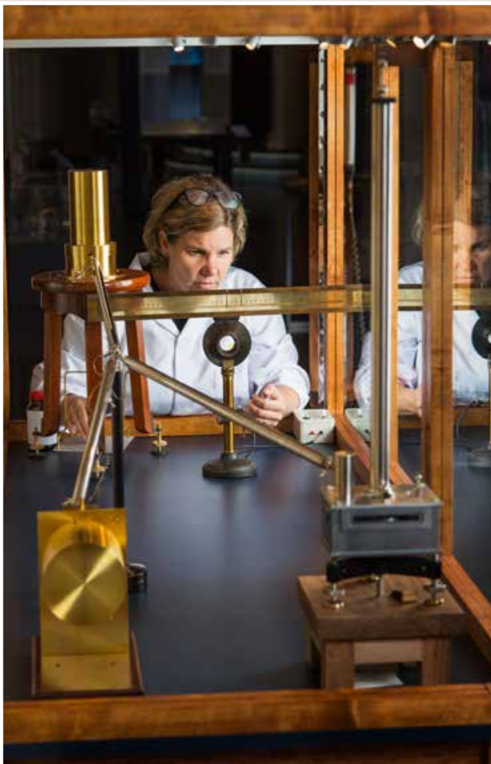
Åsa Husberg at the Nobel Museum uses an exact replica of the original equipment to perform the experiment in which Pierre and Marie Curie managed to measure radioactivity.
