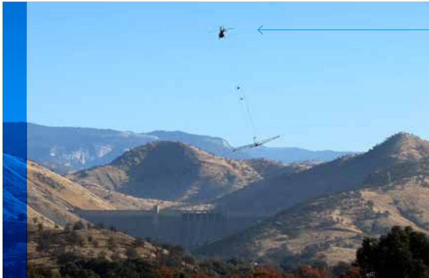
Helicopter carrying an electromagnetic imaging camera to survey the geology in California's Central Valley.
